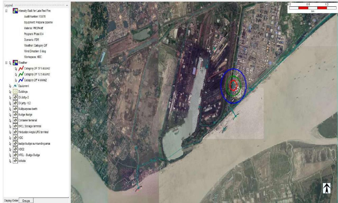
28. Flash fire from Full Bore Rupture of **Propane** pipeline from Oil jetty-I with wind speed **2 m/s** and **F** stability class.
