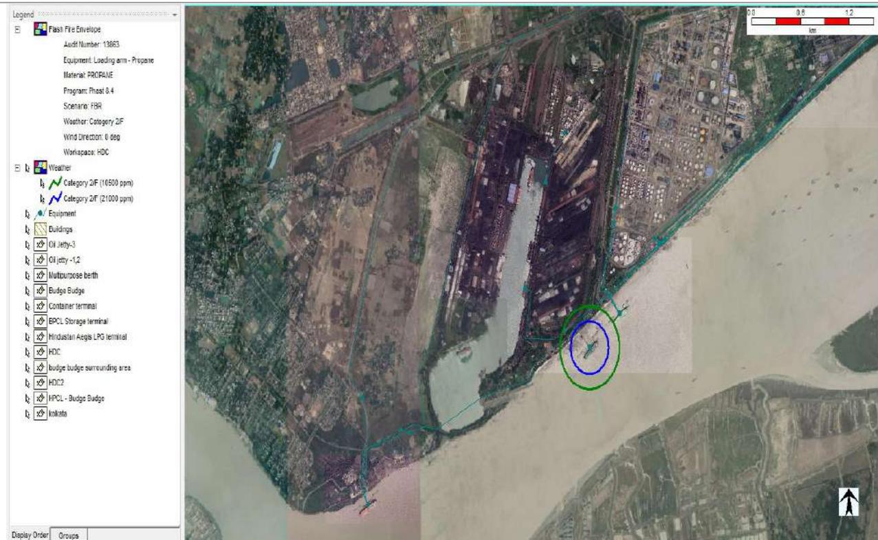
15. Vapour Cloud Explosion from Full Bore Rupture of Propane unloading arm with wind speed 2 m/s and F stability class at Oil Jetty-II (OJ-II).
