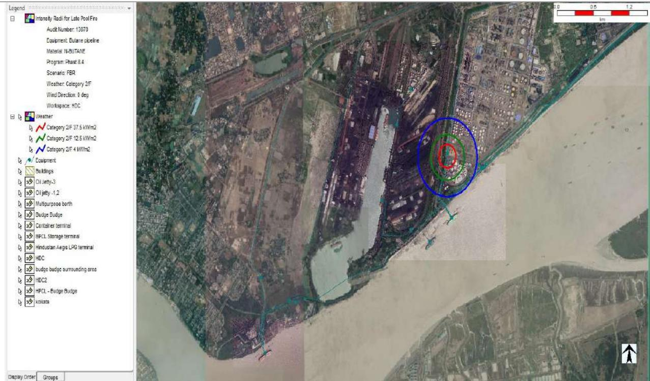
**31. Vapor cloud explosion** from Full Bore Rupture of **Butane** pipeline from Oil jetty-I with wind speed **2 m/s** and **F** stability class.
