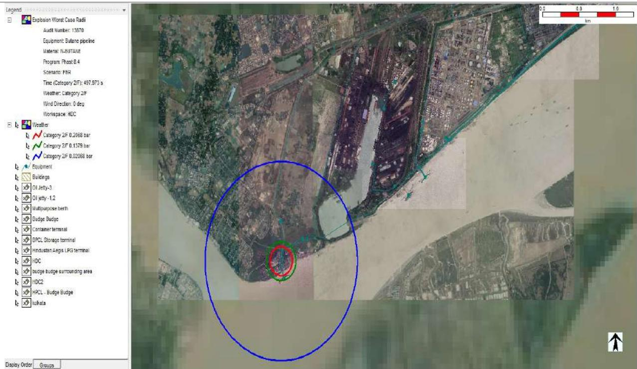
37. Pool fire from Full Bore Rupture of Xylene pipeline from Berth 2 with wind speed 2 m/s and F stability class.
