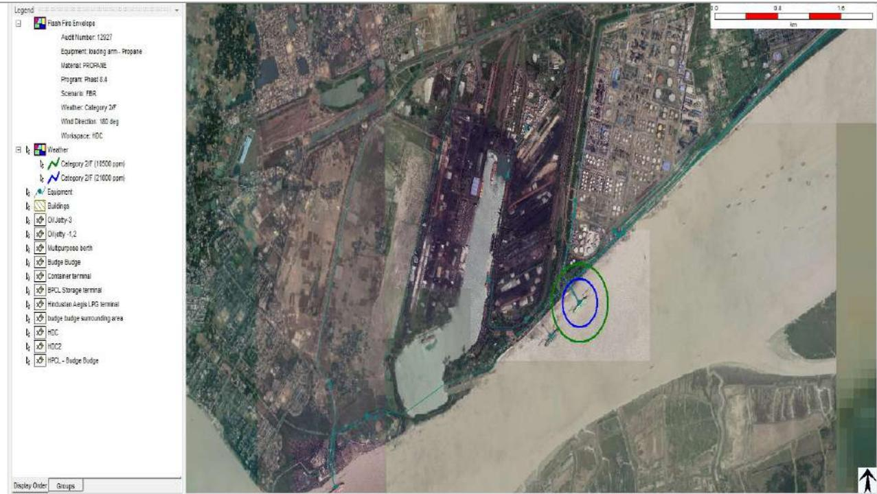
2. Jet fire from Full Bore Rupture of Propane unloading arm with wind speed 2 m/s and F stability class at Oil Jetty-I (OJ-I).
