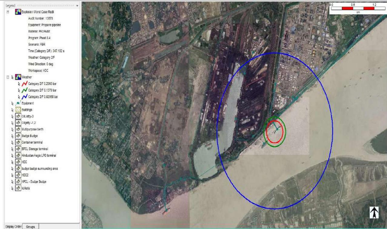
30. Pool fire from Full Bore Rupture of Butane pipeline from Oil jetty-I with wind speed 2 m/s and F stability class.
