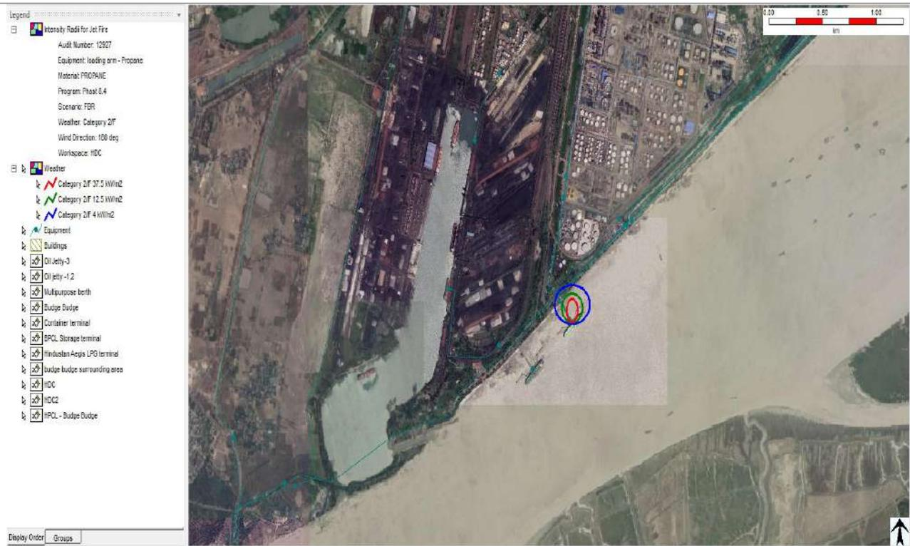
**3. Vapor Cloud Explosion from Full Bore Rupture of Propane unloading arm with wind speed 2 m/s and F stability class at Oil Jetty-I (OJ-I).**
