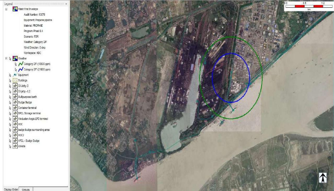
29. Vapour Cloud Explosion from Full Bore Rupture of Propane pipeline from Oil jetty-I with wind speed 2 m/s and F stability class.
