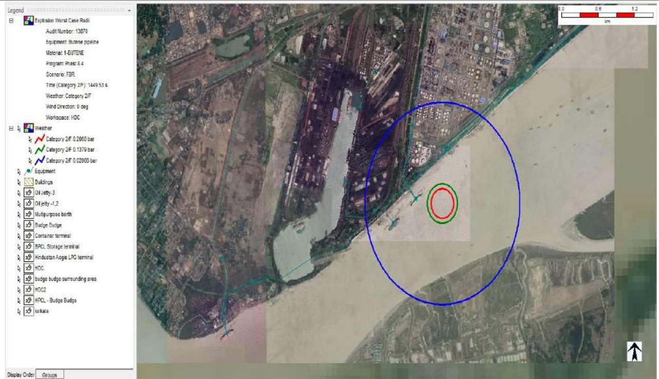
34. Jet Fire from Full Bore Rupture of **propane** pipeline from Oil jetty-III with wind speed 2 m/s and F stability class.
