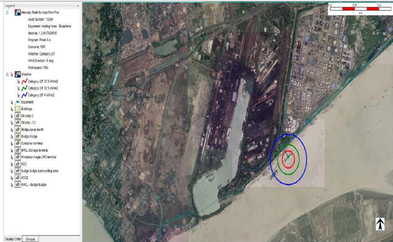
11. Flash fire from Full Bore Rupture of **Butadiene** unloading hose with wind speed **2 m/s** and **F** stability class at Oil Jetty-I (OJ-I).
