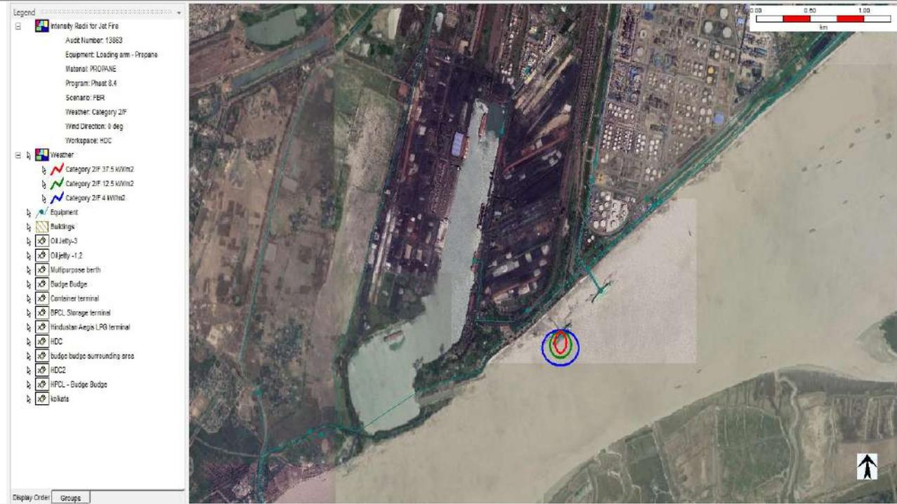
14. Flash Fire from Full Bore Rupture of Propane unloading arm with wind speed 2 m/s and F stability class at Oil Jetty-II (OJ-II).
