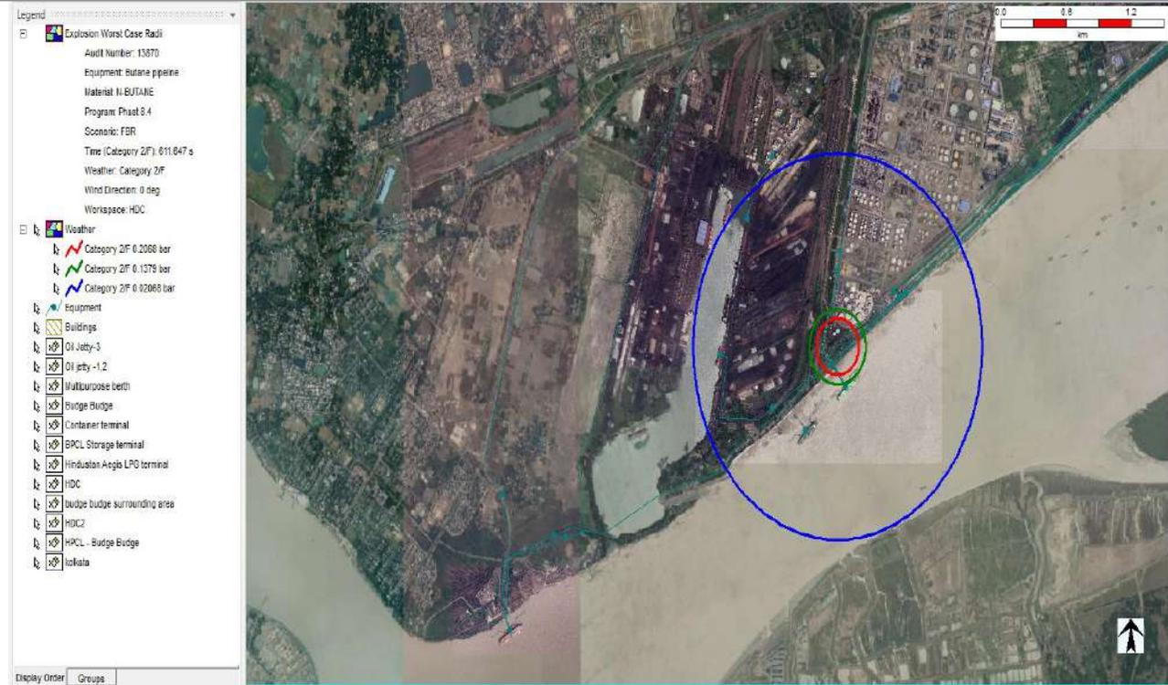
**32. Toxic Dispersion** from Full Bore Rupture of **Ammonia** pipeline from Oil jetty-I with wind speed **2 m/s** and **F** stability class.
