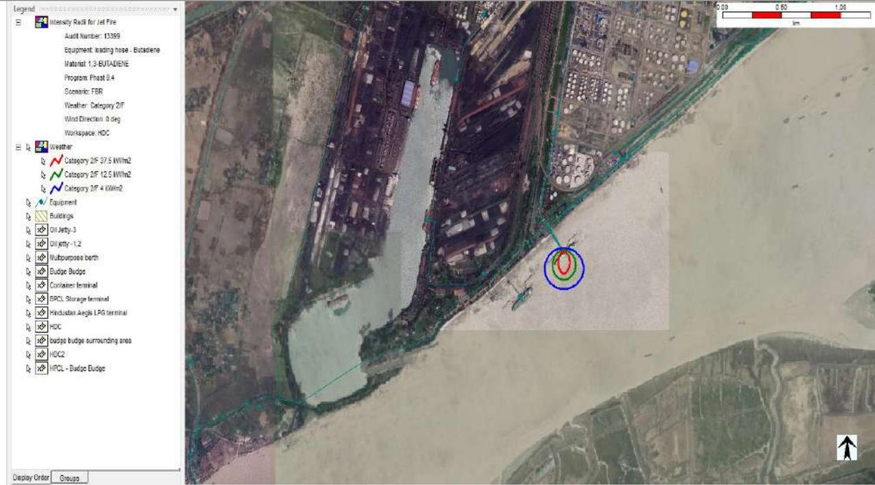
10. Pool fire from Full Bore Rupture of **Butadiene** unloading hose with wind speed **2 m/s** and **F stability class** at Oil Jetty-I (OJ-I).
