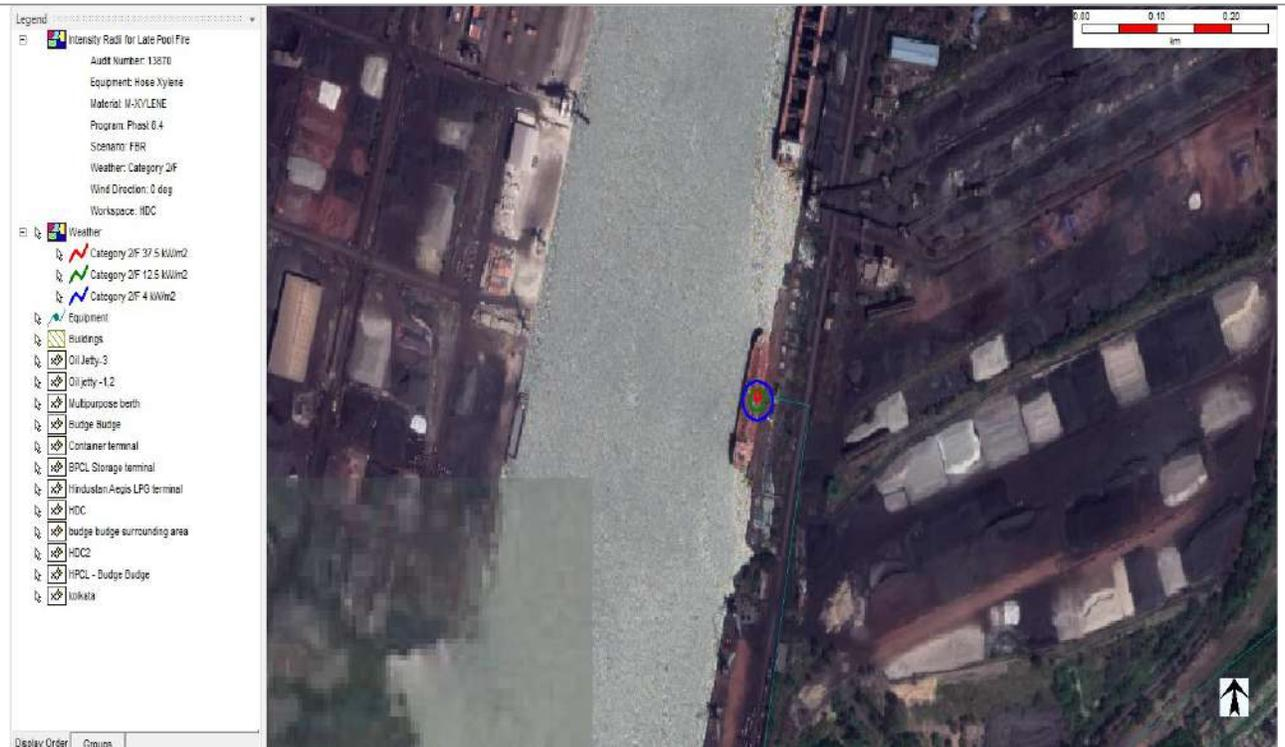
25. Vapor cloud explosion from Full Bore Rupture of Benzene unloading hose with wind speed 2 m/s and F stability class at Multipurpose Berth.
