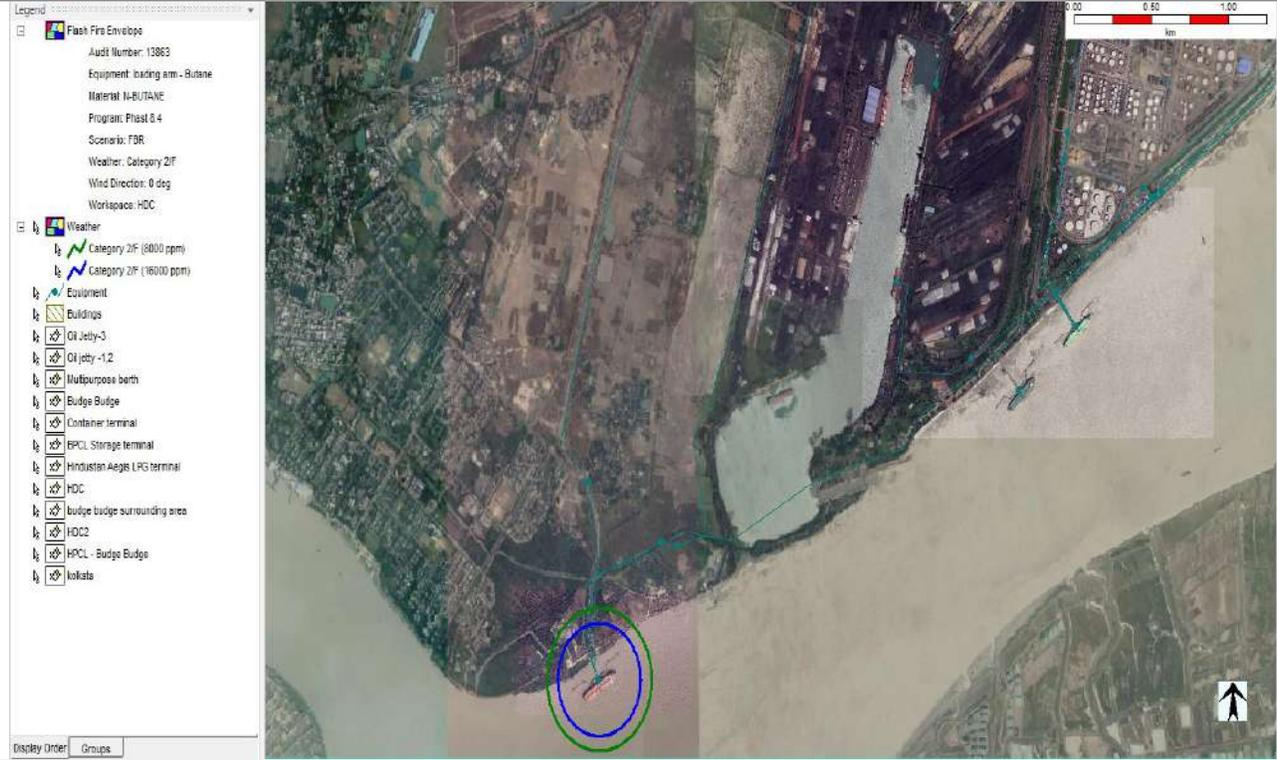
22. Vapor cloud explosion from Full Bore Rupture of **Butane** unloading arm with wind speed 2 m/s and **F stability class** at Oil Jetty-III (OJ-III).
