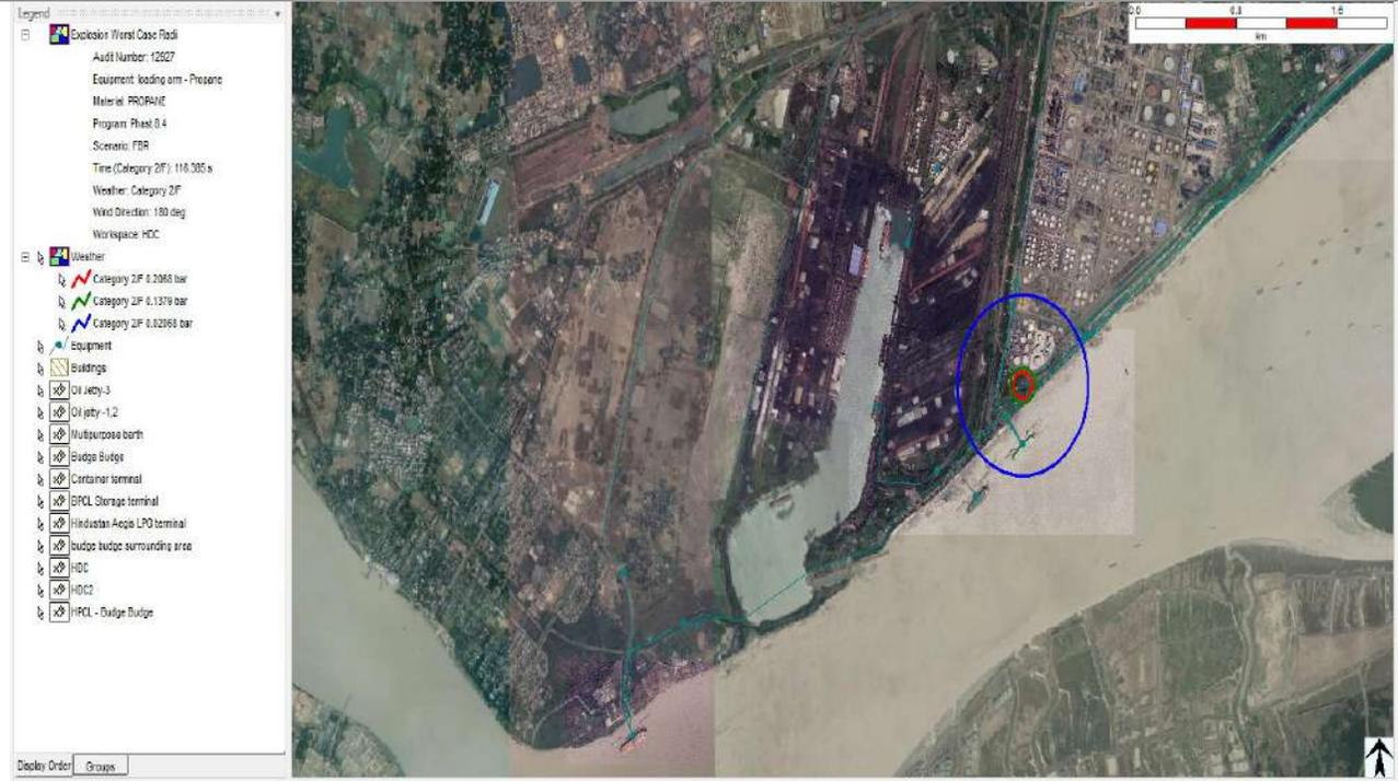
**4. Vapor Cloud Explosion from Full Bore Rupture of Butane unloading arm with wind speed 2 m/s and F stability class at Oil Jetty-I (OJ-I).**
