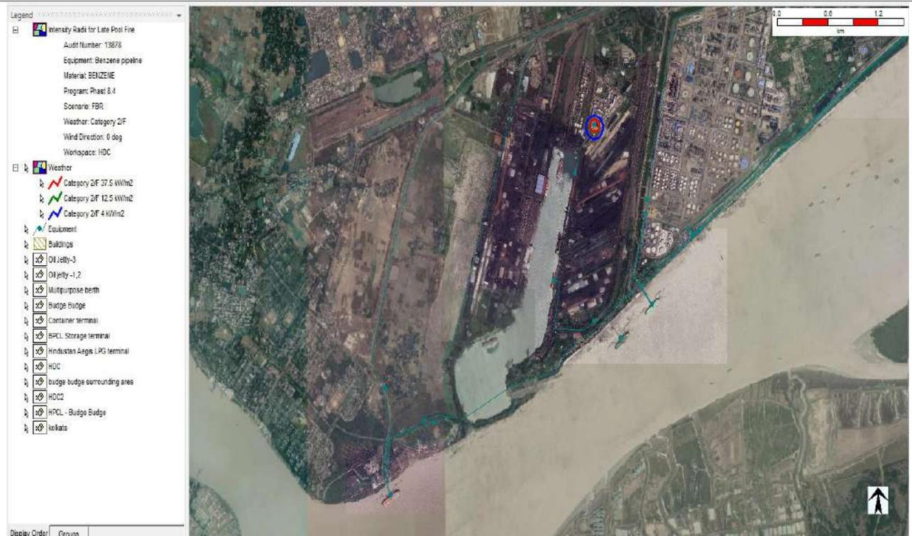
39. Pool fire from Full Bore Rupture of HSD pipeline from Berth 2 with wind speed 2 m/s and F stability class.
