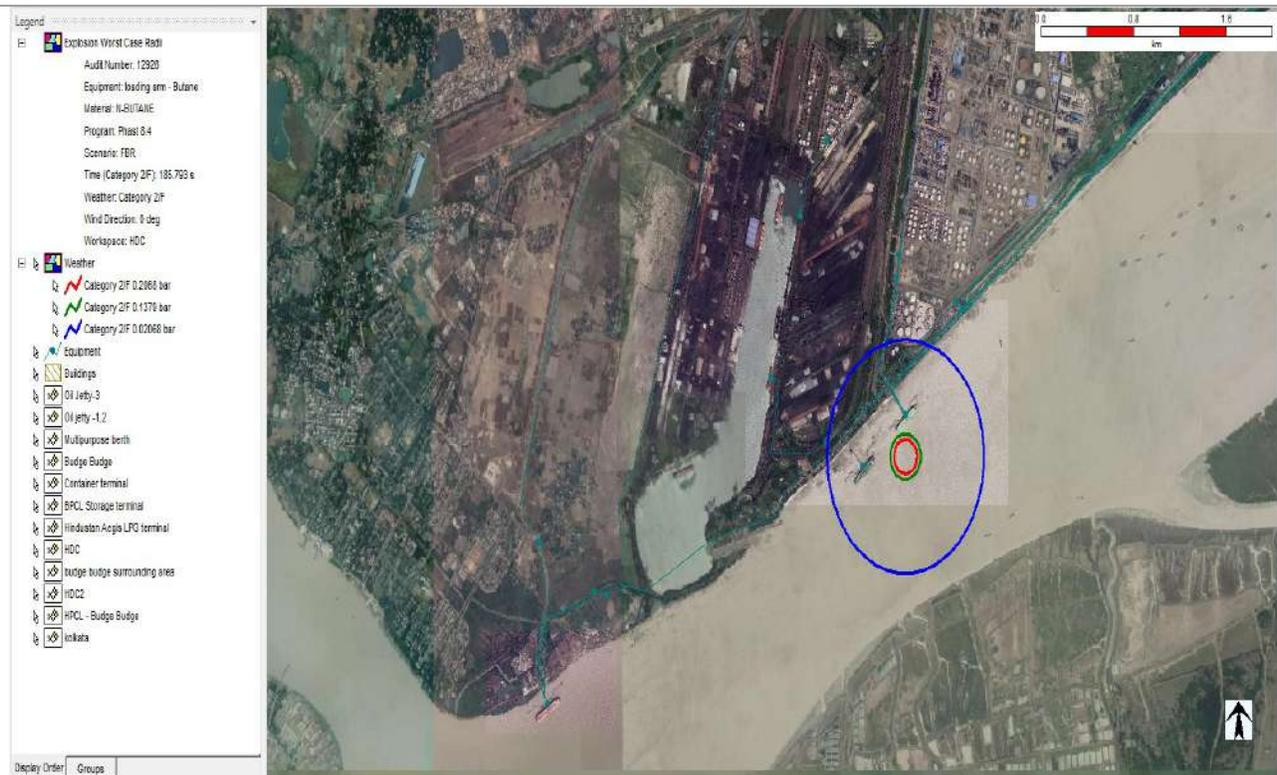
5. Jet fire from Full Bore Rupture of **Butene** unloading hose with wind speed 2 m/s and **F stability class** at Oil Jetty-I (OJ-I).
