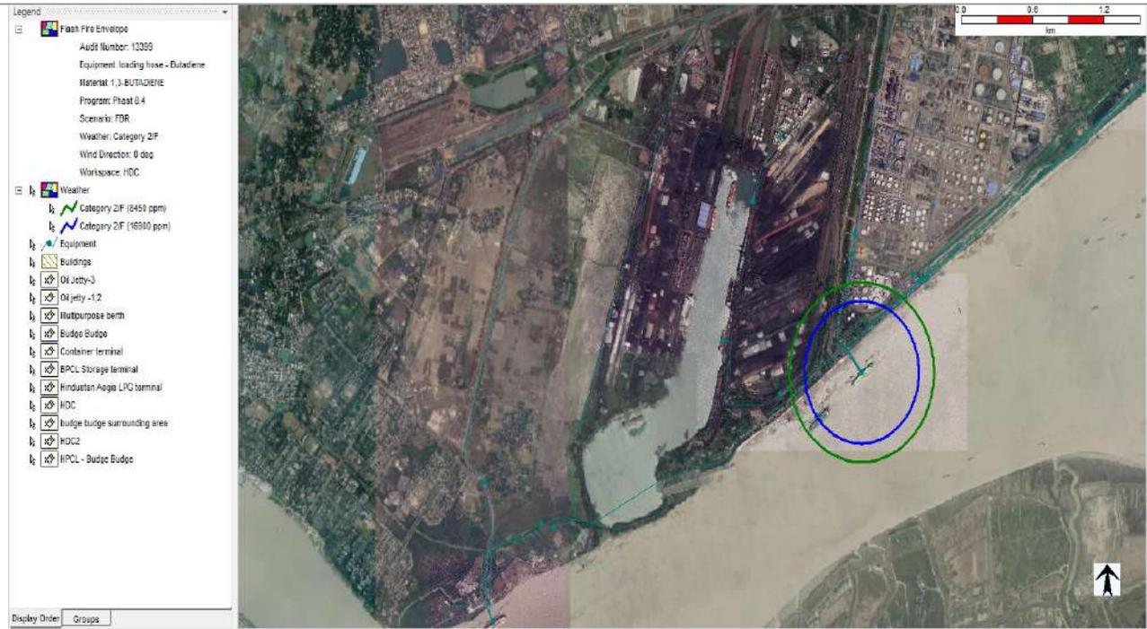
12. Toxic Dispersion from Full Bore Rupture of **Ammonia** unloading arm with wind speed **2 m/s** and **F** stability class at Oil Jetty-I (OJ-I).
