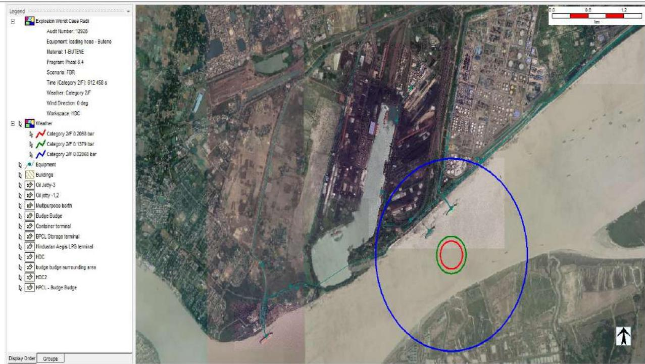
9. Jet fire from Full Bore Rupture of **Butadiene** unloading hose with wind speed **2 m/s** and **F stability class** at Oil Jetty-I (OJ-I).
