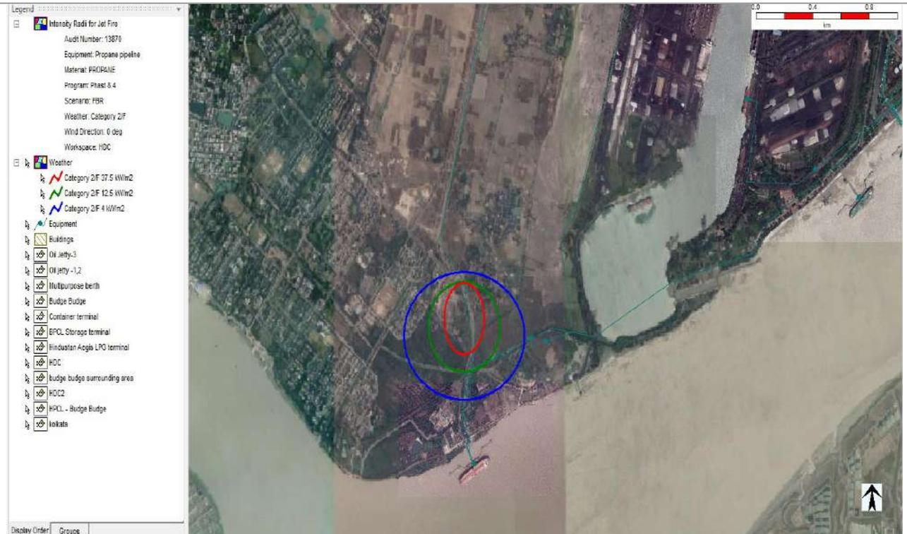
35. Vapour cloud explosion from Full Bore Rupture of **Propane** pipeline from Oil jetty-III with wind speed 2 m/s and F stability class.
