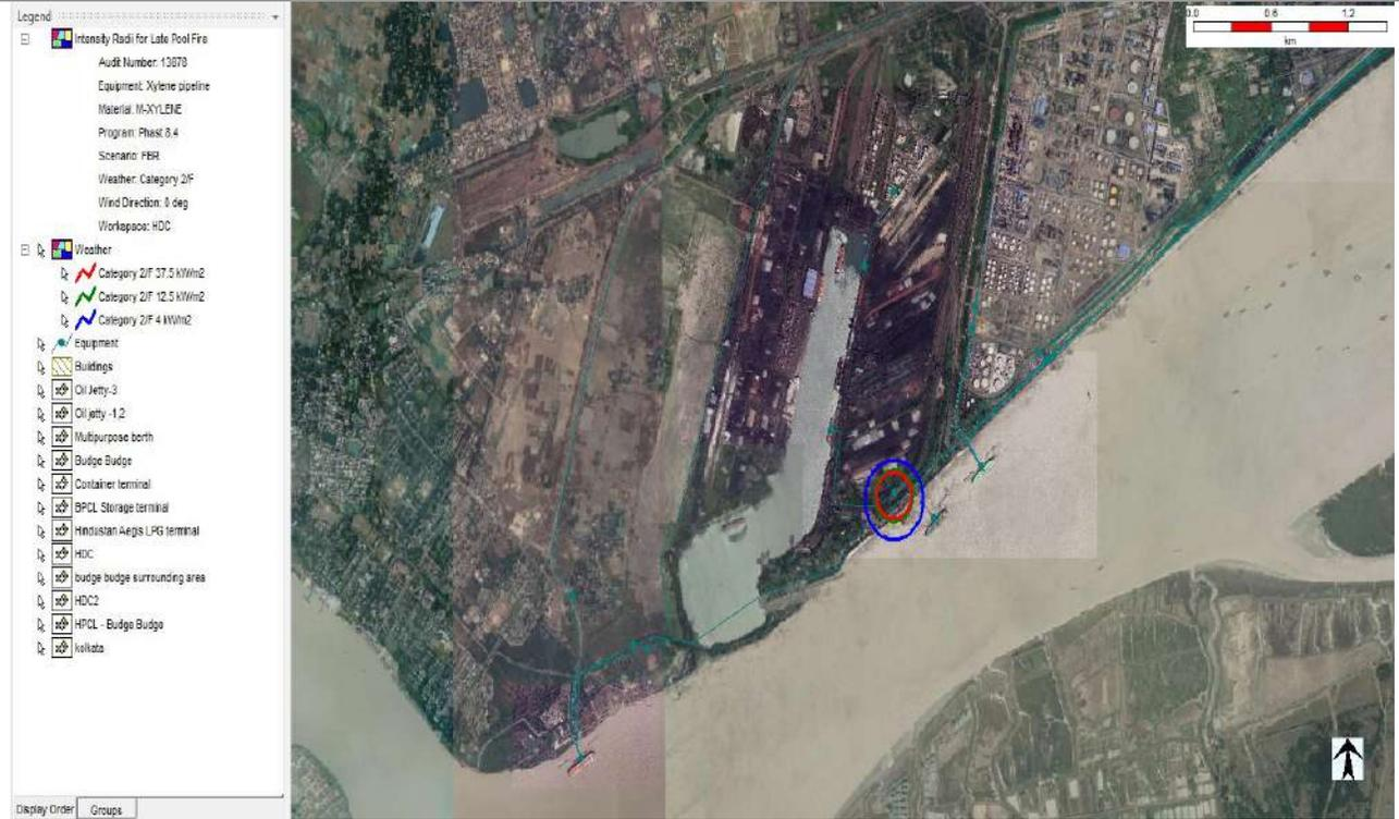
38. Pool fire from Full Bore Rupture of Benzene pipeline from Berth 5 with wind speed 2 m/s and F stability class.
