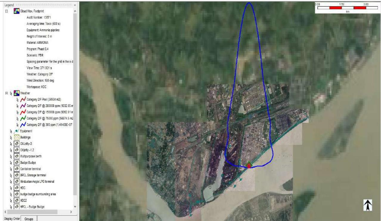
33. Vapour cloud explosion from Full Bore Rupture of **Butene** pipeline from Oil jetty-I with wind speed 2 m/s and F stability class.
