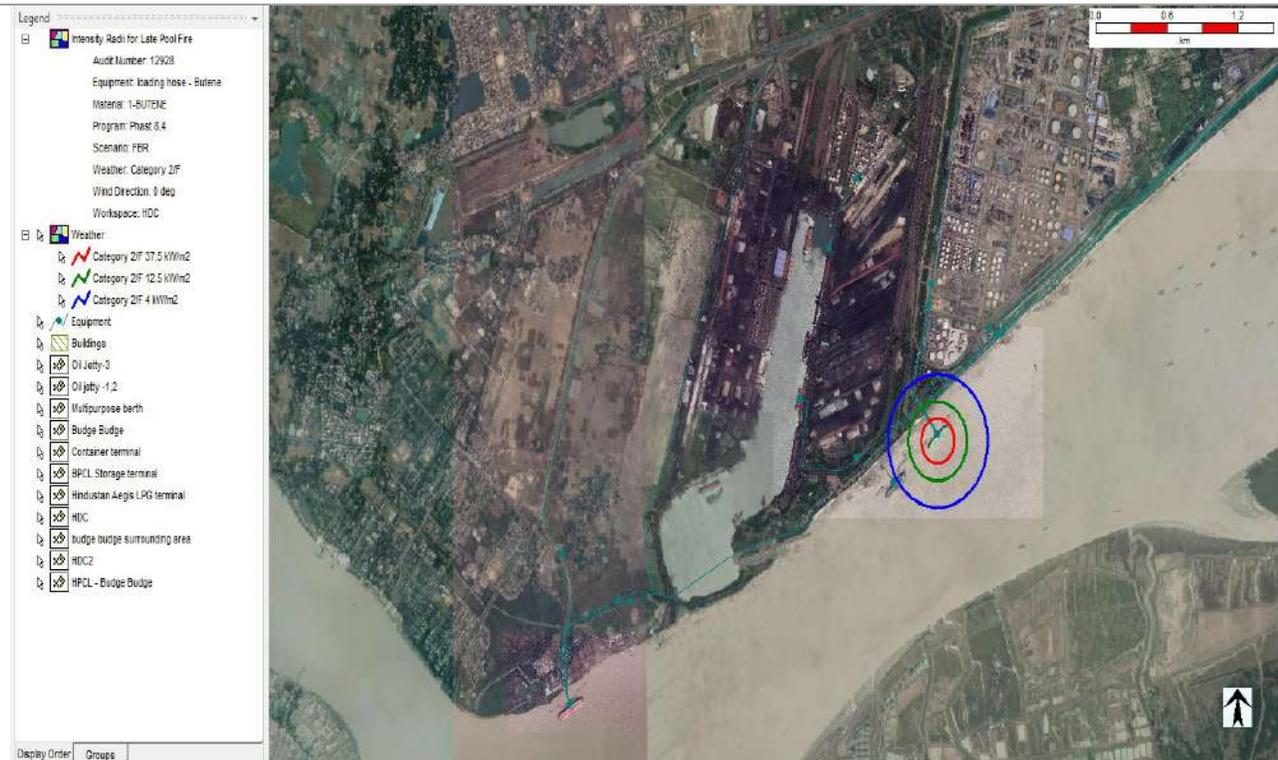
7. Flash fire from Full Bore Rupture of **Butene** unloading hose with wind speed 2 m/s and **F stability class** at Oil Jetty-I (OJ-I).
