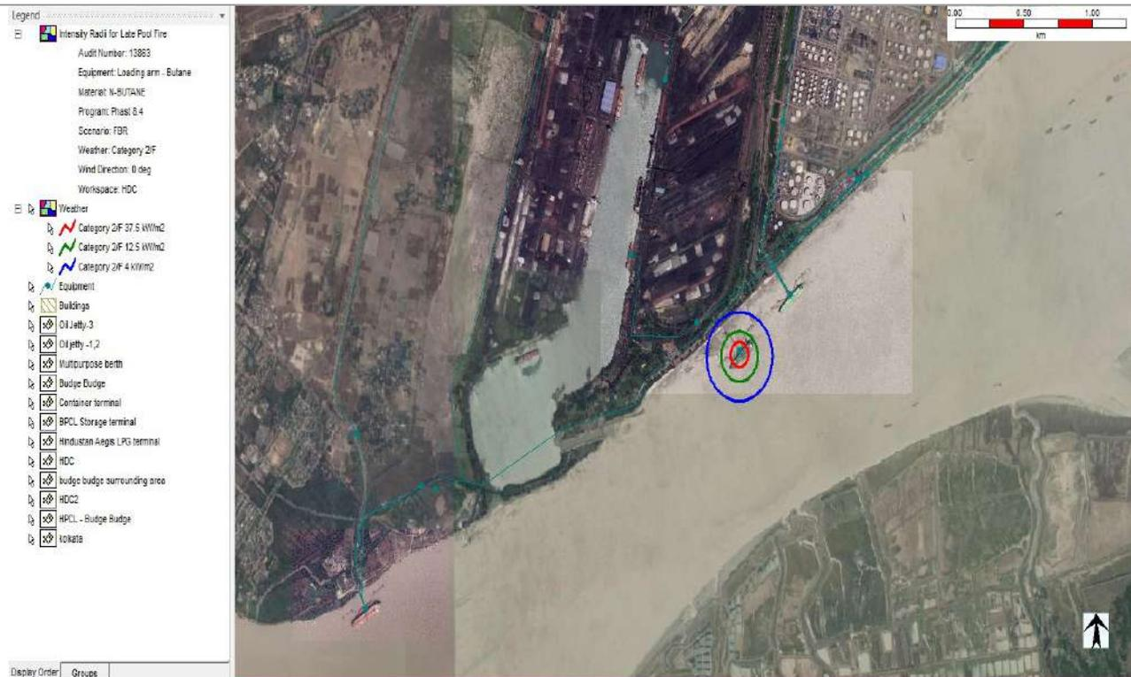
17. Vapor cloud explosion from Full bore rupture of **Butane** unloading arm with wind speed **2 m/s** and **F stability class** at Oil Jetty-II (OJ-II).
