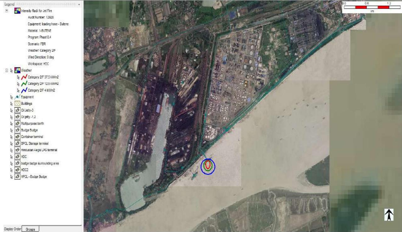
6. Pool fire from Full Bore Rupture of **Butene** unloading hose with wind speed 2 m/s and **F stability class** at Oil Jetty-I (OJ-I).
