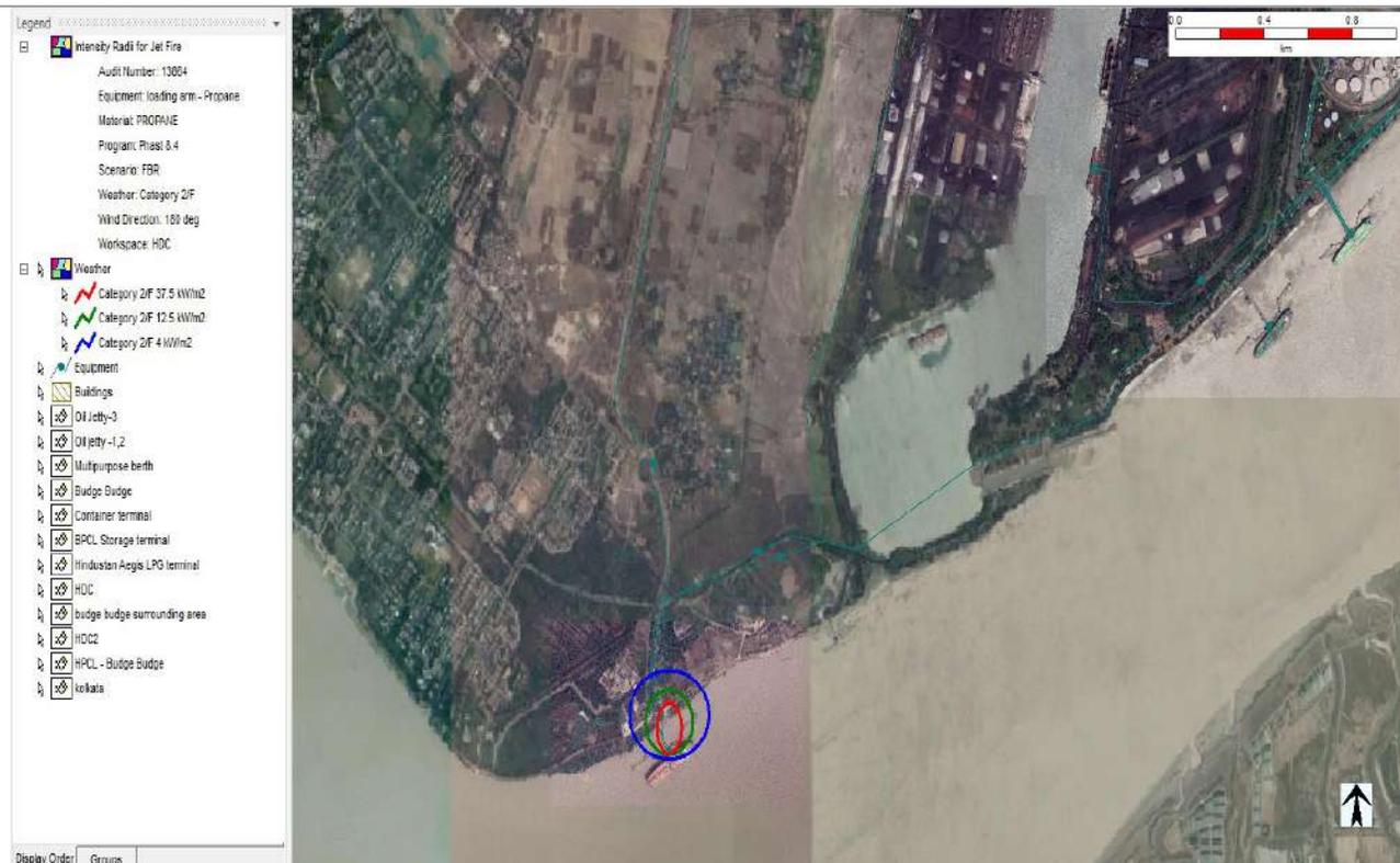
19. Flash fire from Full bore rupture of Propane unloading arm with wind speed 2 m/s and F stability class at Oil Jetty-III (OJ-III).
