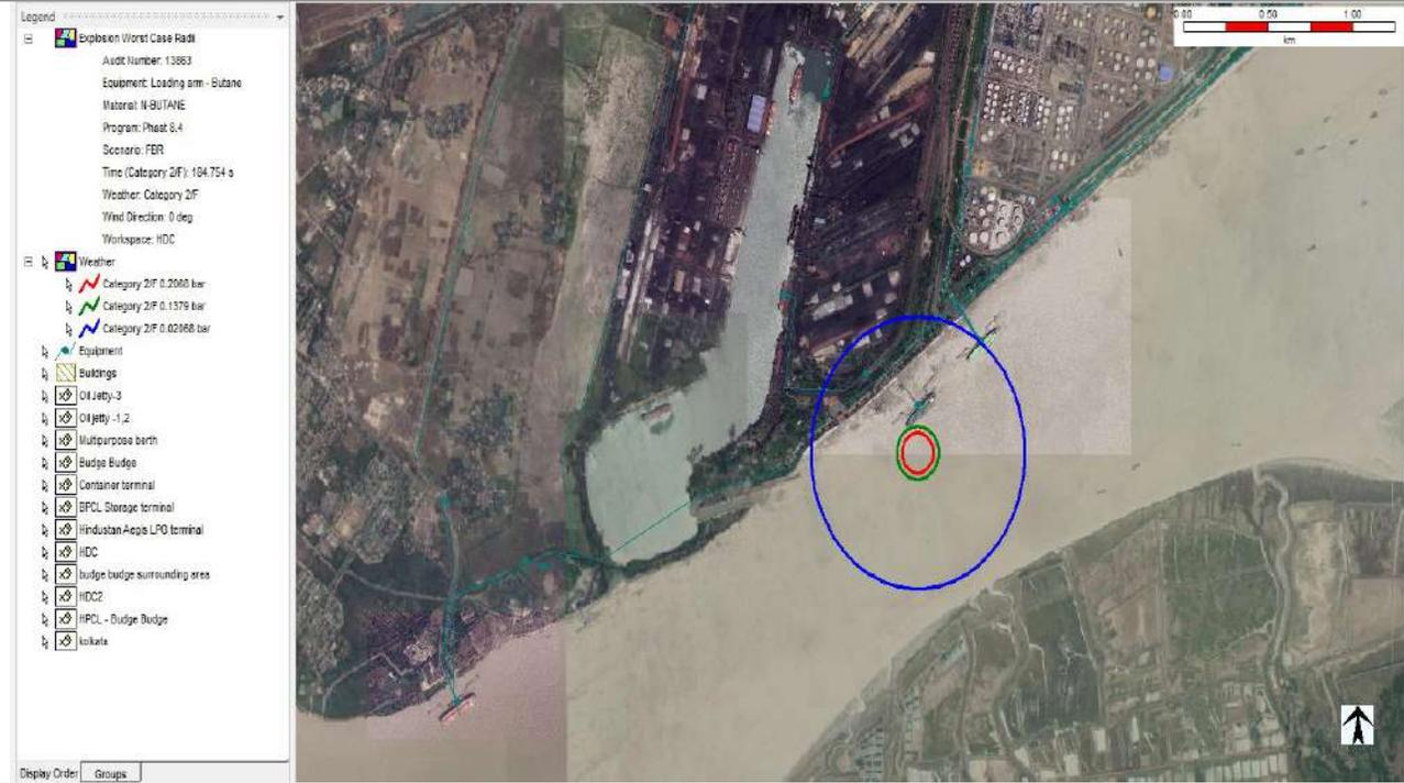
18. Jet fire from Full bore rupture of **Propane** unloading arm with wind speed **2 m/s** and **F stability class** at Oil Jetty-III (OJ-III).
