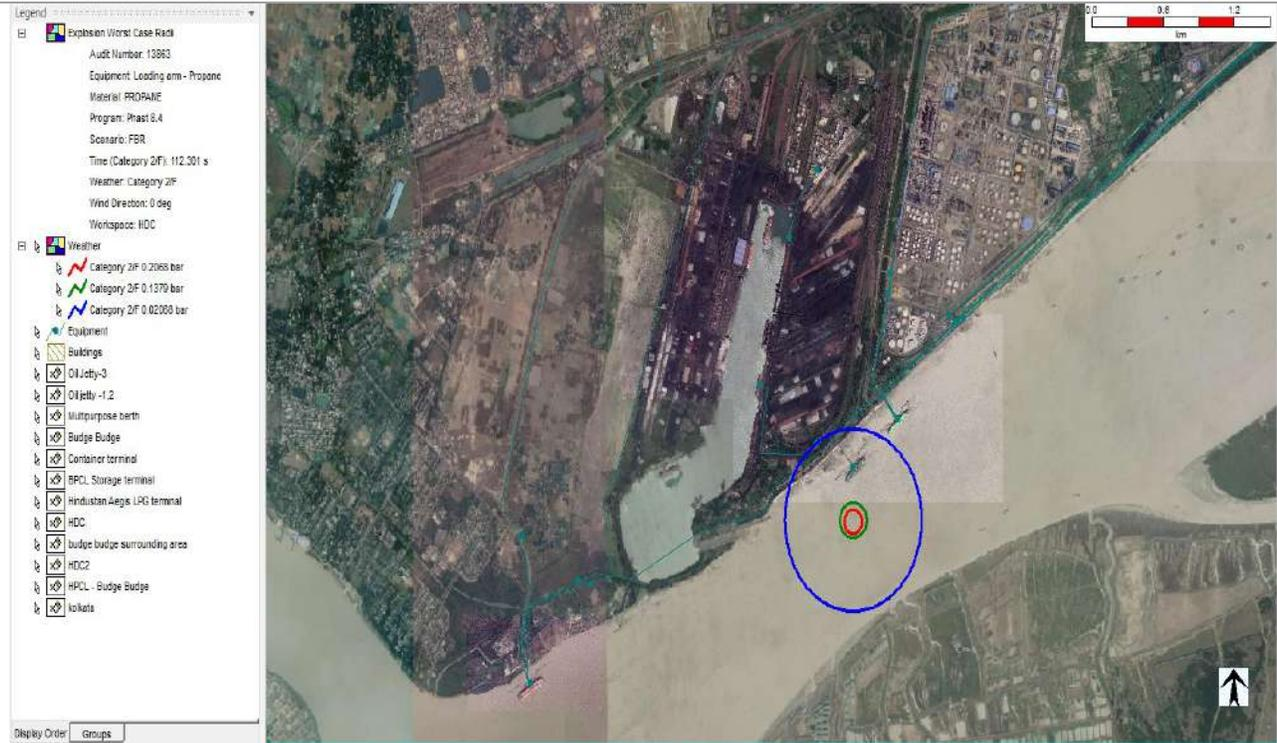
16. Pool Fire from Full Bore Rupture of Butane unloading arm with wind speed 2 m/s and F stability class at Oil Jetty-II (OJ-II).
