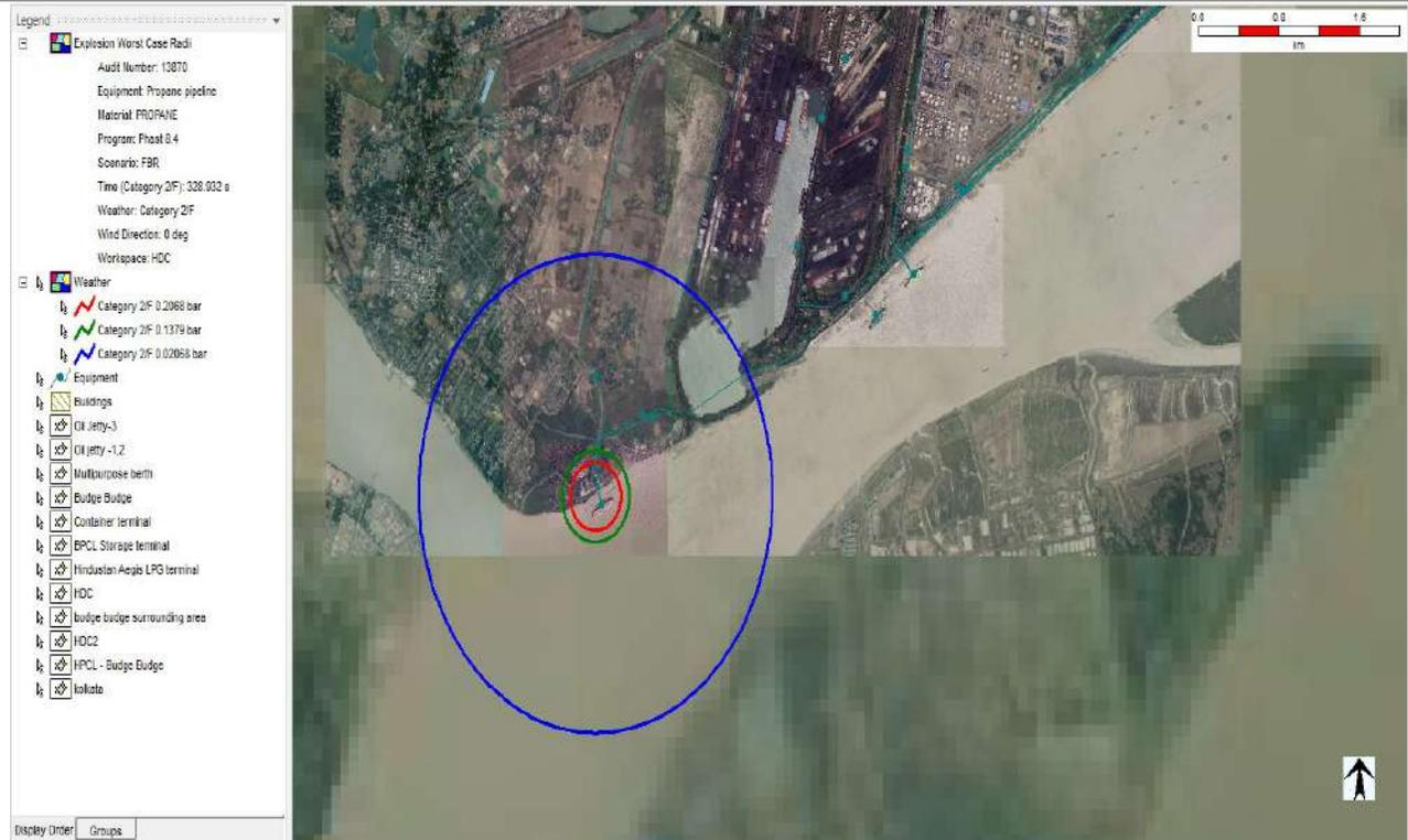
36. Vapor cloud explosion from Full Bore Rupture of **Butane** pipeline from Oil jetty-III with wind speed 2 m/s and F stability class.
